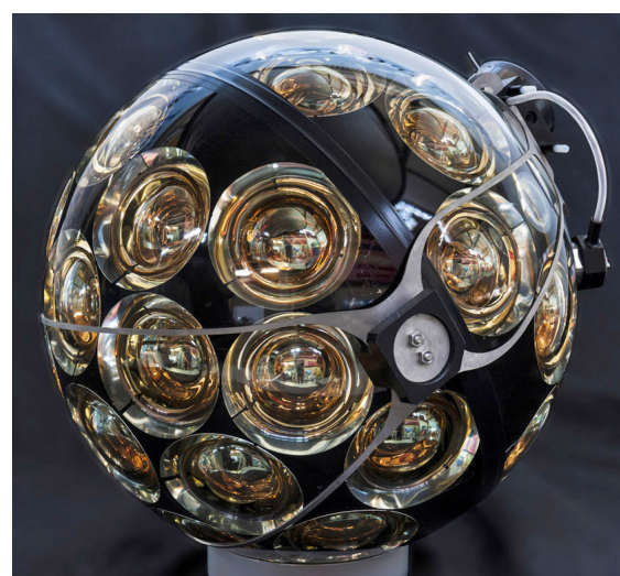
DOM optic module (modelization). © KM3NeT
